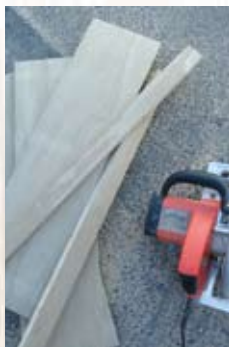
Step one Measure and cut the plywood to the dimensions as listed above.
