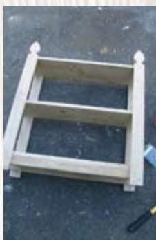
Step six Attach the two remaining pickets to the shelves using PVA glue and nails. Again, use a set square to check that the shelves are at right angles. Allow the glue to dry.
