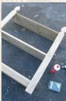
Step five Attach the middle and top shelves to the pickets, as shown, using PVA glue and nails. Ensure the shelves are evenly spaced.
