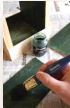
Step four Paint the underside of the roof panels with one coat of Resene Rangitoto. Leave to dry for 24 hours and apply a second coat of Resene Rangitoto.
