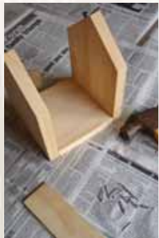
Step one Assemble the sides and base of the bird feeder, fixing with nails provided and exterior PVA glue.
