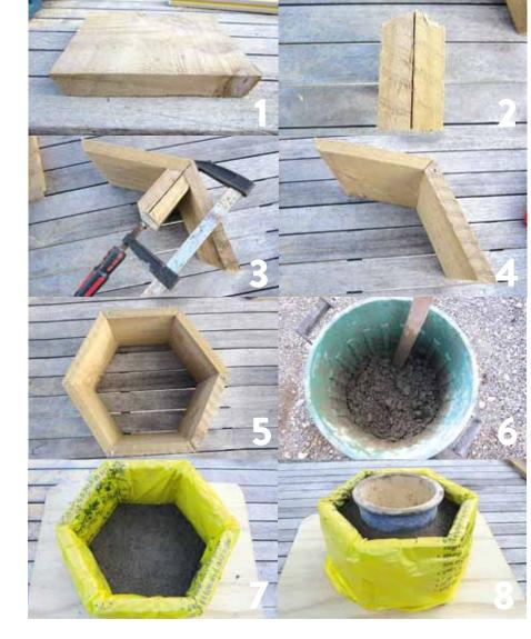
1 Start by making the frames. Hexagons need six sides with 60° angles at each end. Set the drop saw angle to 30°. Cut the first angle, mark 20cm, turn timber and cut second angle. Marking timber at 20cm and reversing each time, cut six pieces.
