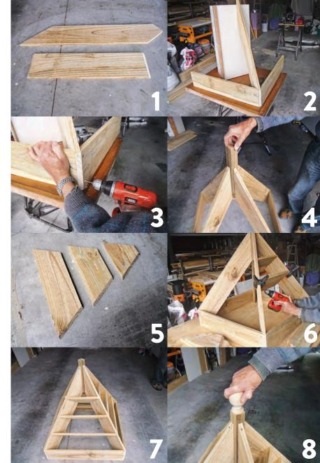
On each 760mm length, cut a 45° bevel at each end. On each 980mm length, cut a 52° angle at one end. At the other end cut two angles – one at 52° and one at 38°.
