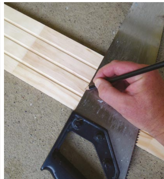
Step 2 Using the back of the saw, as shown, mark cutting lines across the moulding.
