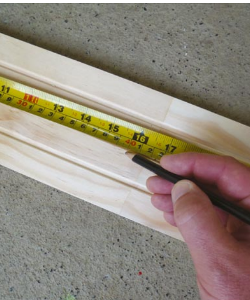
Step 1 Measure two pieces at 400mm and five pieces at 260mm along the length of the wooden moulding.
