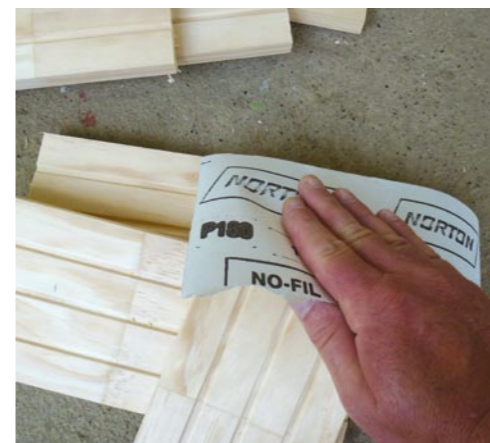
Step 4 Smooth any rough edges with sandpaper.
