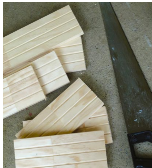
Step 3 Using the lines as a guide, cut the moulding into the seven pieces.
