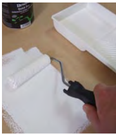
Step three Mask off a 30mm strip around the edge of the board and apply two coats of Resene Zomp, removing the masking tape before the second coat has dried.
