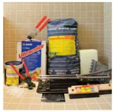
You'll need: Flexible tile adhesive; notched adhesive trowel; reinforced fibre mesh; brush and waterproofing system; grout (coloured to match tiles); tiles; plumb line; sponge; plastic spacers; flat rubber stamp; fine-tooth scraper; rotary tile cutter and/or straight nipper or wet saw; silicone; corking gun.
