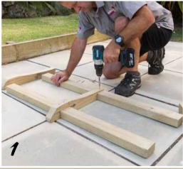
1. Start with the seat. Make the frame for the seat base, using our photograph as a template, or use straight pieces if preferred. Sand any cut edges. Pre-drill the holes so that the screws can counter-sink for a neater and more comfortable finish, and use the glue for extra strength.
