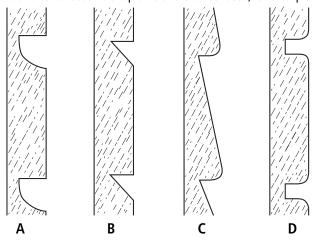
Type **C** is by far the most desirable profile for painting, and on most weatherboard houses the bottom angle is bevelled.
